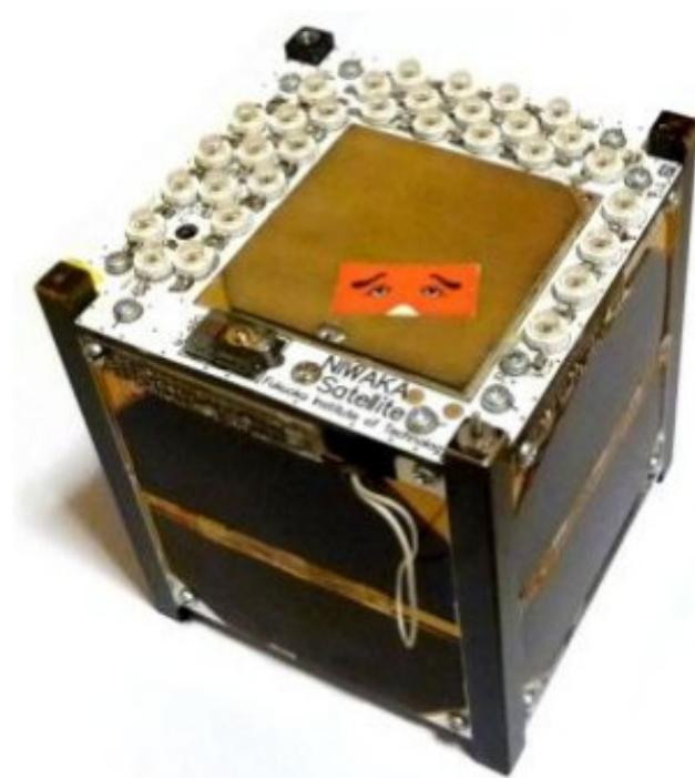
Figure 1-3: Photograph of FITSAT-1 showing a patch antenna (brown) surrounded by LEDs [3]
