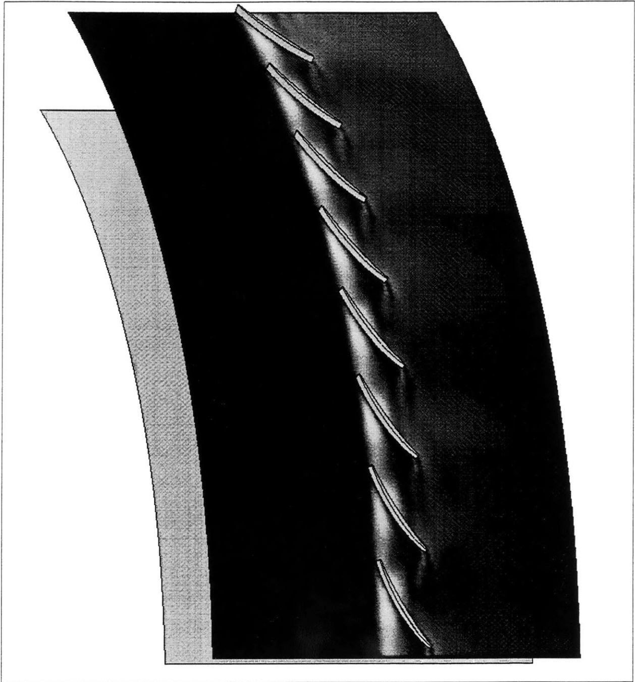
Figure 5.8: Vorticity contour at 8% immersion of the E^3 compressor with 3.0% clearance (Time = -5.9)
