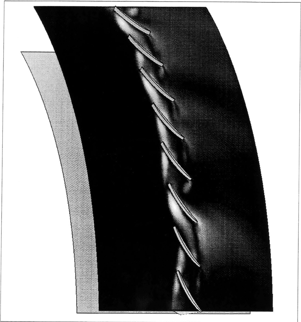
Figure 5.9: Vorticity contour at 8% immersion of the E^3 compressor with 3.0% clearance (Time = -4.1)
