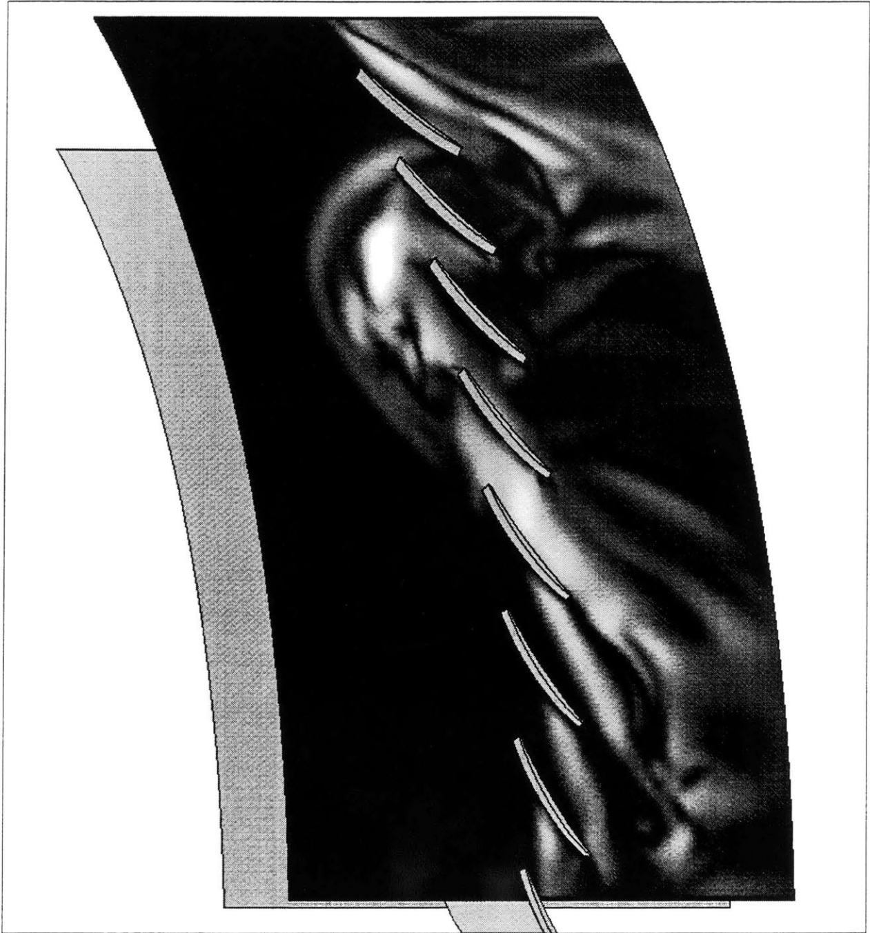
Figure 5.11: Vorticity contour at 8% immersion of the E^3 compressor with 3.0% clearance (Time = 1.0)
