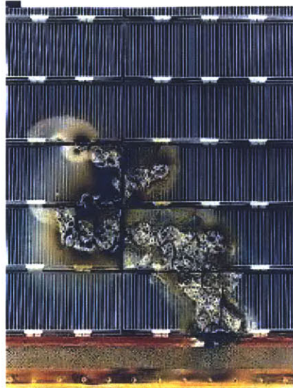
Figure 1-1: Damage to the solar array on the ESA EURECA mission due to a sustained arcing event from surface charging. Image Source: Ferguson and Hillard (2003) [41].
