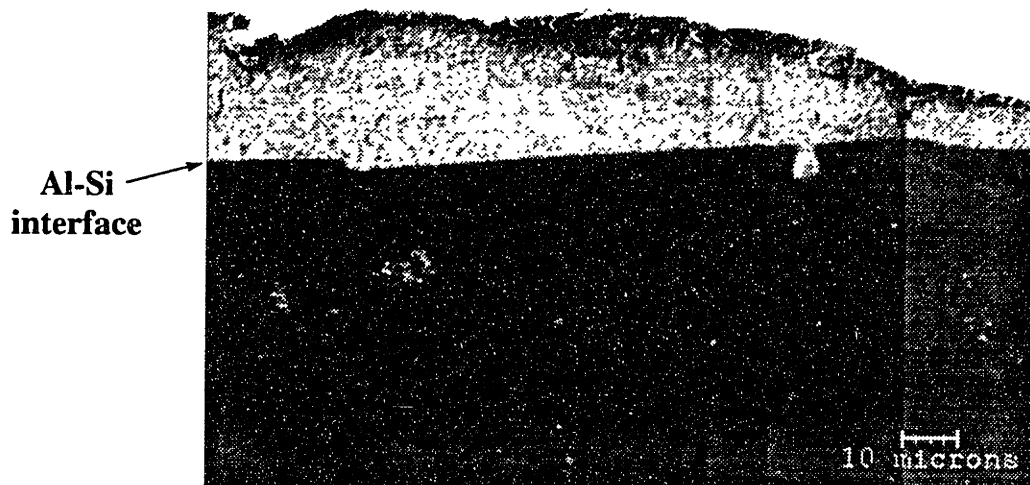
Figure 2.4 SEM micrograph showing a cross sectional view of the contact area on a (111) wafer. Processing was at 850°C for 30 minutes. Notice step formation and pitting along (111) planes.
