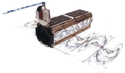
Figure 2-15: Image of a Dove CubeSat from Planet [6]
