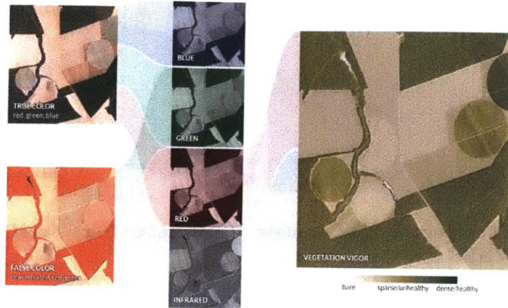
Figure 2-14: The four imaging bands on the Dove CubeSats are combined into one picture [63]
