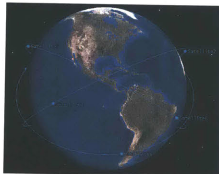
Figure 1-1: A Walker constellation of 9 satellites, three satellites evenly spaced per plane, three planes with evenly spaced RAANs, all planes at a 30^\circ inclination.
