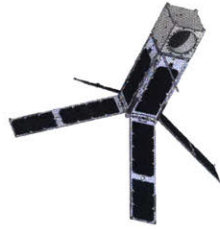
Figure 2-7: MicroMAS-2 CAD illustration. The upper 1U of the CubeSat contains the rotating microwave radiometer.
