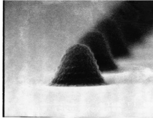
Figure 3-3. (a) Bell shape photoresist dots. (b) The shape has no difference without hard bake process.
