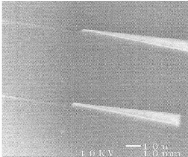
Figure X-4. SEM images of the unclad tapers defined by etching of \text{Si}_x\text{O}_y\text{N}_z stack with \text{CHF}_3 . The images reveal excellent alignment of the stack and the waveguide. The sidewall is smooth and stack profile angle is 78 degree.
