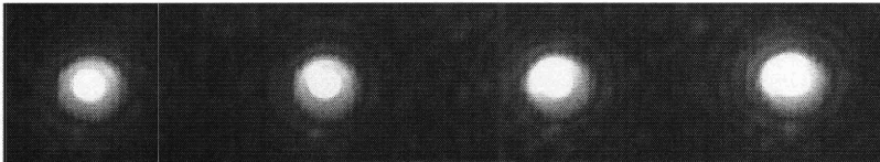
Figure V-3. Optical attenuator of 3.3 OD was used to avoid saturation of the detector with input light from a 1x4 MMI.
