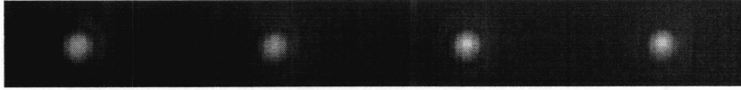
Figure V-6. Near field output of 1x4 MMI ridge structures at w=8, 10\ \mu\text{m} with silicon-rich \text{Si}_x\text{N}_y core. The outputs are uniform across the 4 ports.
