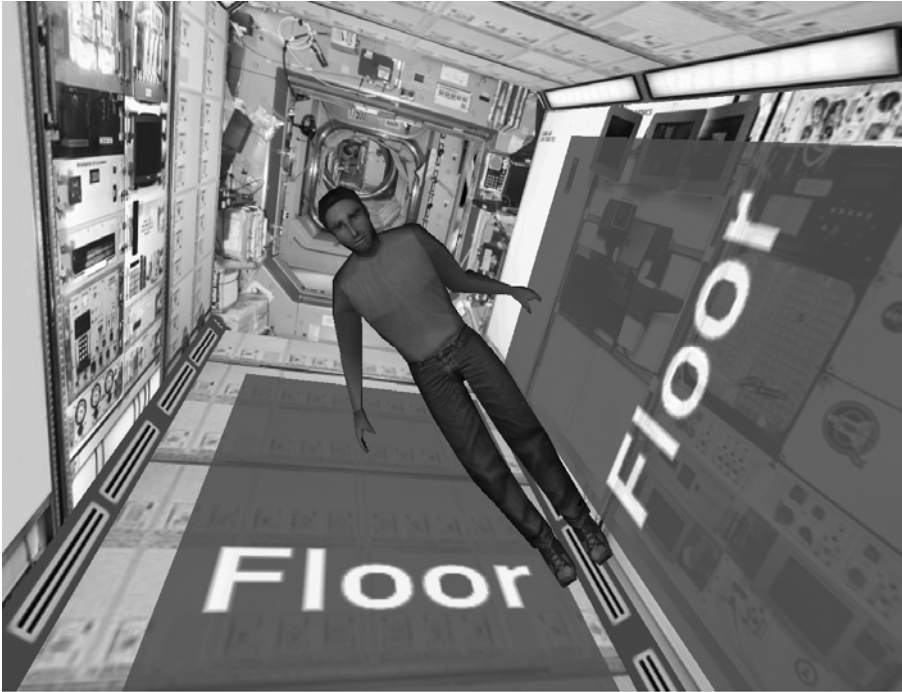
Figure Error! No text of specified style in document.-9. VRI in the ISS US Laboratory module. The equipment and labeling on the true floor and ceiling are oriented 90 degrees counterclockwise from those on the true walls and floor. The square cross section of the module means the major physical axes of symmetry are also 90 degrees apart. When a crewmember floats in this body orientation, which surface is perceived as a floor depends on visual attention. VRIs due to such ambiguities can only be prevented by attending to learned landmarks.
