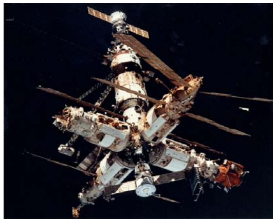
Figure Error! No text of specified style in document.-4. Russian Mir Space Station. In this picture, the Core module is behind, pointing upwards. The Priroda module is to the left, also attached to the central node module, and opposite the Kristall and the orange Shuttle docking
