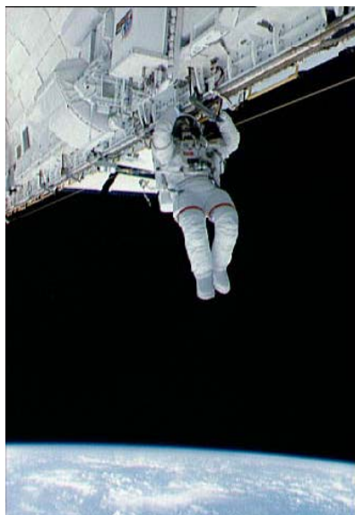
Figure Error! No text of specified style in document.-3. Floating inverted in Shuttle payload bay can cause EVA Height Vertigo (NASA photo)
