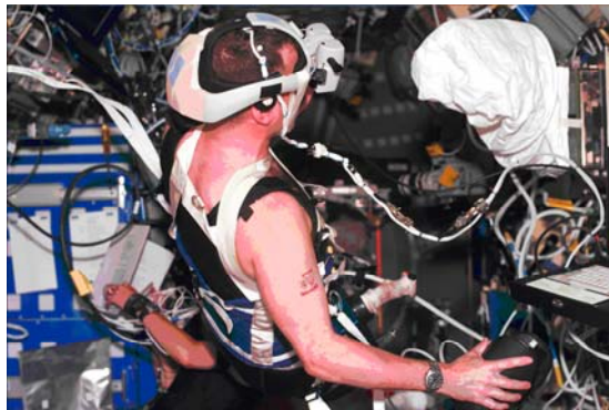
Figure Error! No text of specified style in document. -6. 1998 Neurolab Shuttle mission experiments on individual differences in visual orientation and shape perception. (Oman et al, 2003). The head mounted display provided controlled visual stimuli in the otherwise cluttered and busy laboratory.
