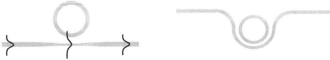
Figure 8.16 – Methods of increasing the coupling between the bus and ring – shrink the waveguide width to expand the mode in the vicinity of the ring (left) or wrap the waveguide around the ring (right).
