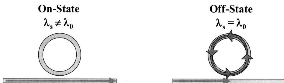
Figure 8.15 – Ring modulator On and Off States where \lambda_s is the signal wavelength and \lambda_0 is the resonant wavelength of the ring.
