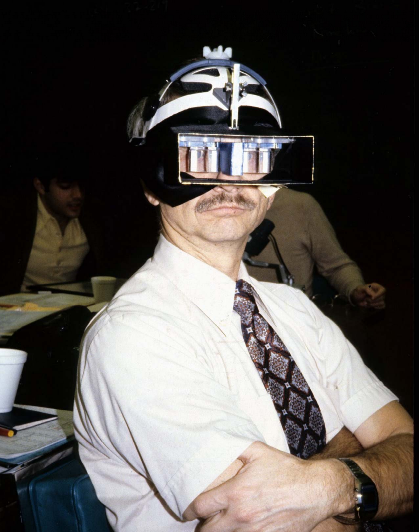
Skylab/Spacelab MS Owen Garriott, prism goggle motion sickness symptom recognition training MIT Feb 1979
