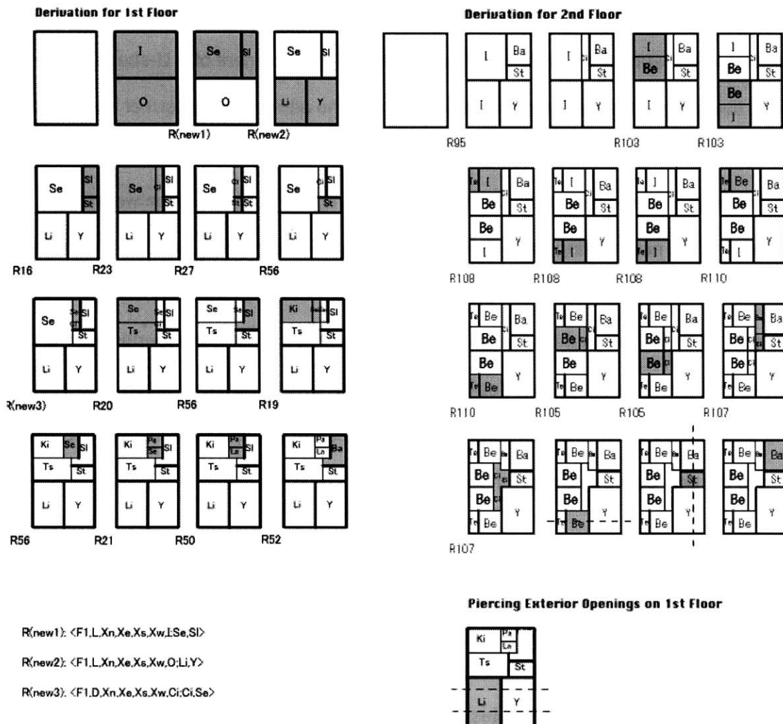
Figure 6.36 - The derivation of design C2 S2 II presented by its design team in the final presentation. Rule numbers do not match those in Figure 5.19 because the rule numbering system was changed after the experiment.
