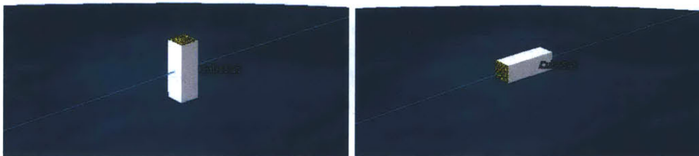
Figure 1-9: Illustration of case study “vertical” (left) and “horizontal” configuration. White surfaces indicate solar cell coverage
