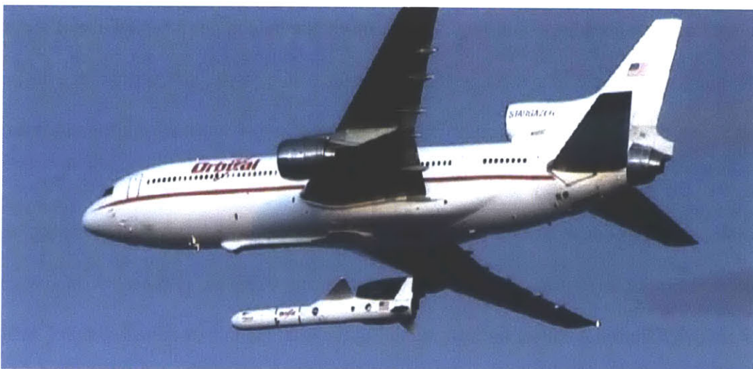
Figure 1.1 —The Orbital Sciences' Pegasus launch vehicle dropped from its carrier aircraft. Image from http://www.nustar.caltech.edu/about-nustar/launch-vehicle
