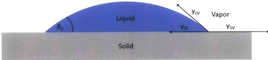
Figure 3-1: Young's Contact Angle: Young's angle is determined by the equilibrium of the three relevant surface tensions on a smooth surface.
