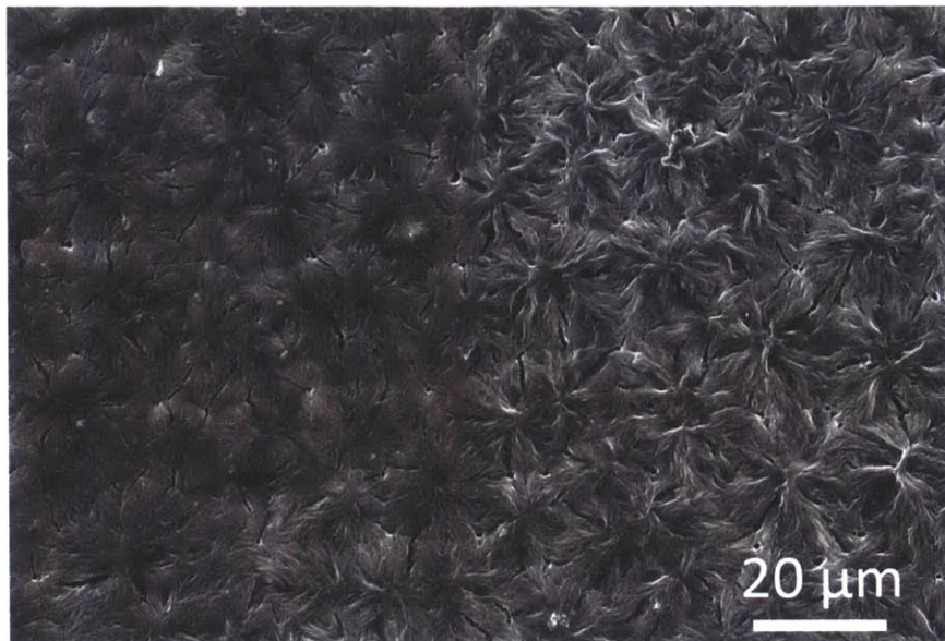
Figure 6-12: Alternative polymer structures on collector electrode: Polymer structures containing radial striations and interesting grain boundaries were observed in some regions of the collector. Later experiments suggest this may result from electro-spray of solvent over deposited fibers.
