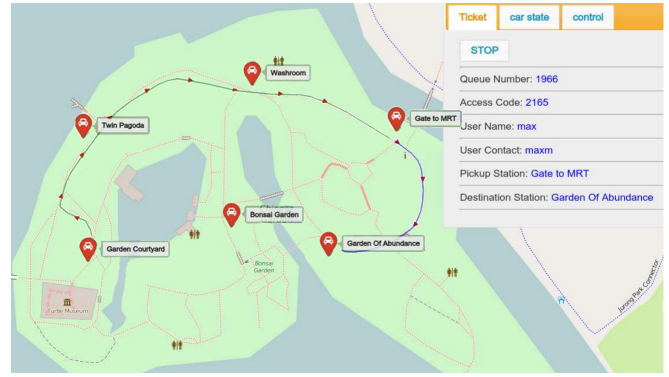
Fig. 10: In-vehicle GUI. The vehicle is currently at Garden Courtyard . The green path represents the route R_{veh;pick} , and the blue path represents the route R_{pick;drop} , which the passenger intends to travel
