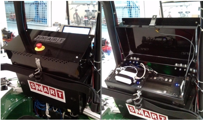
Fig. 6: Computer rack with protective cover. Shown open (right) and closed (left).
