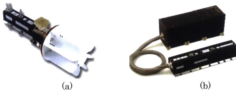
Figure 22. L-3 Communications Electron Technologies, Inc. TWTA devices: a) Ku-band TWT [Menninger et al. , 2013] and b) V-band TWTA [Robbins et al. , 2012]
